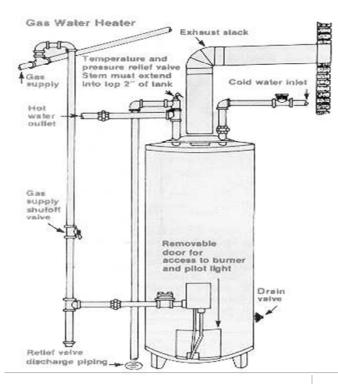
Important Safety Note: Hot water will drain from the line connected to the relief valve when you open it. Have a bucket handy to catch the water. According to the Uniform Plumbing Code, a pipe should be connected to the pressure relief valve, extending down along the side of the tank to within six inches of the floor. This extension pipe prevents the spraying of hot water when the valve is released or if a malfunction were to occur.
