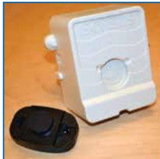
The TouchPad reader shown in the foreground will be covered with the SmartPoint meter reading device.
